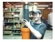
6. Take the new cartridge out of the box and check. Clean grooves if needed.
