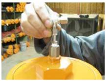
10. Install the 1/4" stainless tubing into the top location of the 90-degree elbow and secure the tubing in place with a 9/16" wrench.
