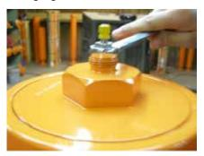
Once the valve is removed, check the condition of the threads in the loading valve port. If necessary, use a <sup>1</sup>/<sub>2</sub>"-20 NF tap and a light lubricant to restore the threads to proper condition.
