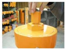
2. Remove the valve stem core from the charging valve.
