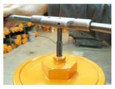
Lightly coat the threads of the <sup>3</sup>/<sub>4</sub>" adapter in the LLA assembly with grease.
