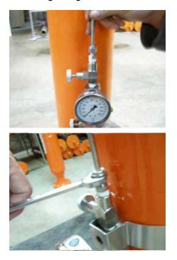
18. Align the tubing with the bleeder valve and label.
