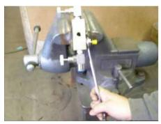
15. Install the pressure gauge into the front of the stainless body as shown. Tighten securely using a 1/2" wrench.
