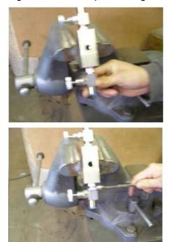
14. Install the lower loading valve into the stainless body at the location shown. Tighten securely with a 3/4" wrench.
