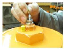
3. Release any pressure present in the stabilizer by loosening the charging valve port using a 5/8" wrench and gently loosening the upper nut at the bottom of the charging valve.
