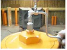
11. Place Teflon tape on the threads of all remaining LLA components.
