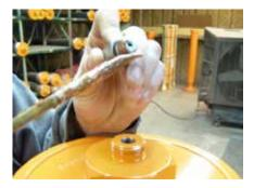
7. Install the LLA adapter in the previous valve port and tighten snugly with a <sup>3</sup>/<sub>4</sub>" wrench.
