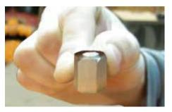
Wrap the threads of the 1/4" tubing adapter and then install the tubing adapter into the 3/4" adapter previously installed in step 7. Use a 7/16" wrench to properly tighten the tubing adapter.
